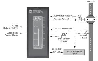
Draft Control General Arrangement \*Not required for "floating" point draft control applications
